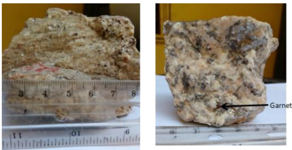
Figure 3: Hand specimen samples revealing quartz, pink alkali feldspar, muscovite and garnet.
