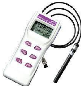
Figure 2: Electrical conductivity meter
