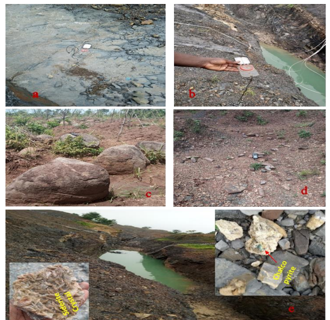
Figure 12: Field Photographs of Ore Veins and Intrusion (a) Indurated shale with quartz veins, Mining Field in Mkpuma-Akpatakpa (b) Mining Field at Mkpuma-Ekwoku, (c) Igneous Intrusive < 300 m from Pb-Zn Site (d) Old cored sample of Igneous Intrusive at (e) Pb-Zn veins trending NW-SE and N-S at Akpatakpa.
