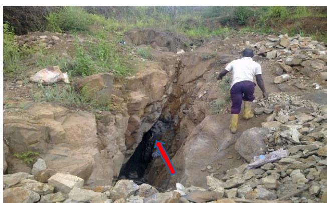
Figure 14: A Sulphide vein (Red arrow) within the Dolerite Sill Ore at Greenfield Mine 4 Ishiagu (Picture was taken by Isabella (Isabella, 2020)).
