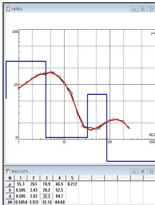
Vertical electrical sounding curve for Okirika
