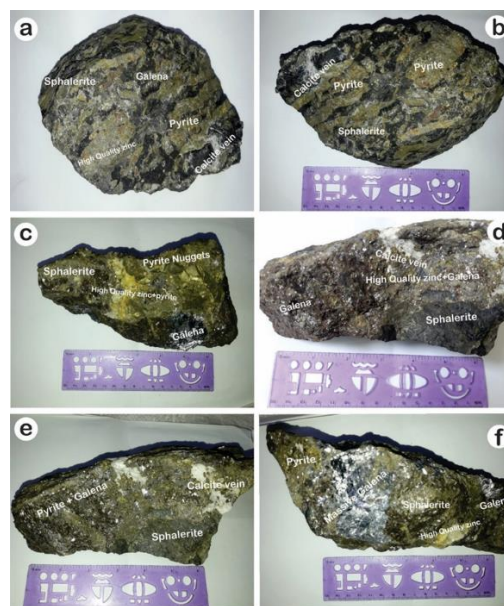
Figure 6: Photographs showing ores samples of Duddar deposit. (a), (b) A massive sulfide ore composed of pyrite and fine-grained sphalerite, locally with dark mudstone fabrics. (c) pyrites nuggets with high grade zinc ore with galena, (d) high grade galena with calcite vein and fine grain sphalerite matrix, (e) pyrite and galena with calcite vein are presented, (f) massive galena with high grade zinc chunks and fine grain pyrite Matrix are presented.
