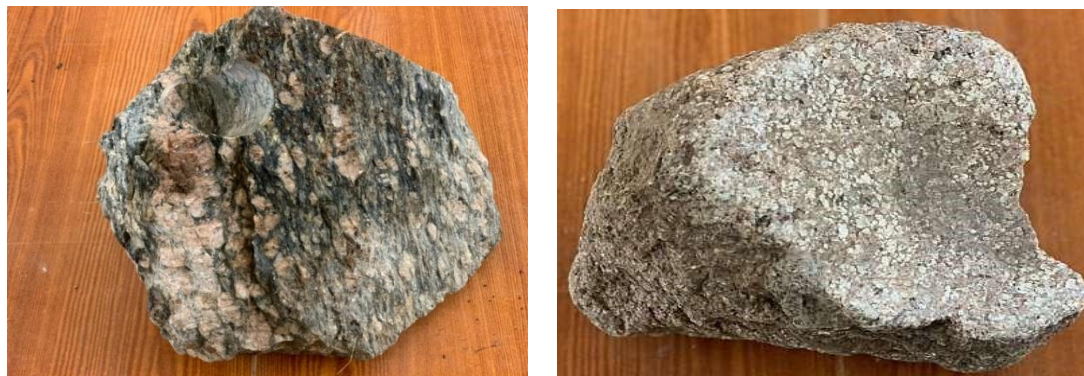
Figure 4: Megascopic descriptions of rocks of coarse-grained minerals of feldspars, quartz, biotite and hornblende sampled at: (A) Green Valley; and (B) Akrofu in Volta Region of Ghana.
