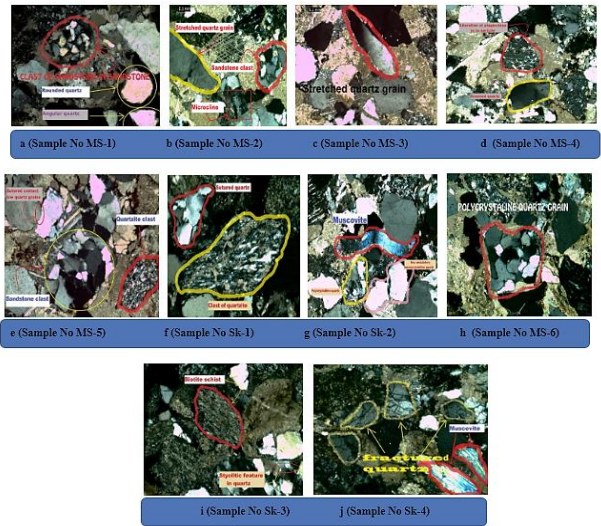
Figure 4: Shown the quartz grain of Sandstone of Rawalpindi Group (a) sub-angular and rounded (b) sub-rounded quartz grains. stretched (c, d), strained (e), sutured (f, g), monocrystalline (h) polycrystalline (i, j) (PPI; 10X).
