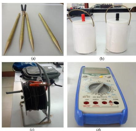
Figure 4: Equipment used for the SP measurement: (a) copper stake electrodes; (b) electrodes of Cu/CuSO 4 porous pots; (c) wire reel; (d) multimeter.
