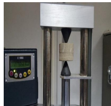
Figure 17: Point Load Test
